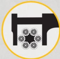
CORRECT WAY TO MEASURE WITH CALIPERS
