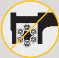
INCORRECT WAY TO MEASURE WITH CALIPERS
