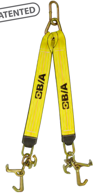
Low Profile V-Strap with R, T & Mini J Hooks PART # LENGTH WLL LP11-8CLU 2' 5,400 lb LP11-8CLU30 2 1/2' 5,400 lb LP11-8CLU36 3' 5,400 lb LP11-8CLU72 6' 5,400 lb
