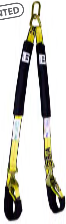
Low Profile V-Strap for Exotic Vehicles PART # LENGTH WLL LP11-EC44 4' 4" 4,700 lb HVLP11-EC44 4' 4" 4,700 lb
